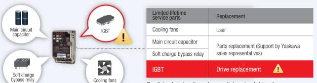
Predicts deterioration of essential parts of drives!
