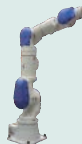
MOTOMAN-SIA30D Payload: 30 kg
