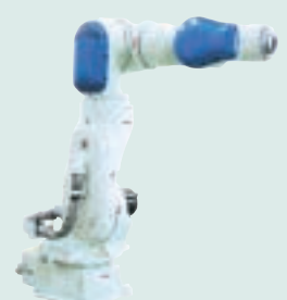
MOTOMAN-SIA50D Payload: 50 kg
